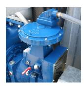
**Priming system** Diaphragm pump, air-cooled, water-resistant and oil-spillage free. Air capacity of 50 m<sup>3</sup> per hour.
